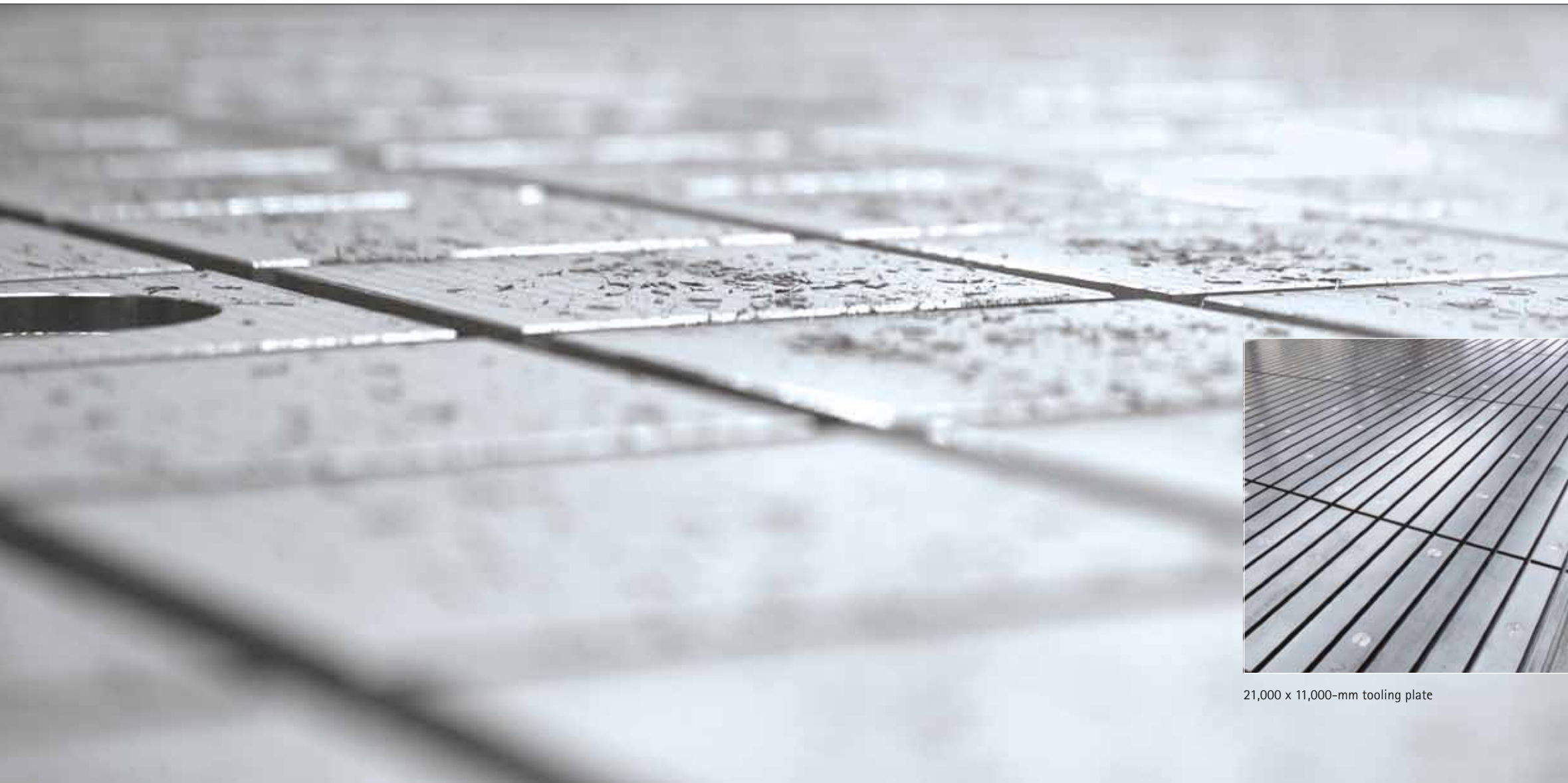
Tooling plate in a moving column milling machine
