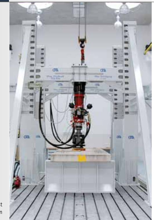
Tooling plate for static tests
