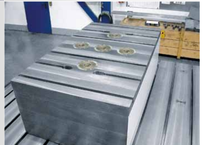
Clamping towers with zero-point clamping system
