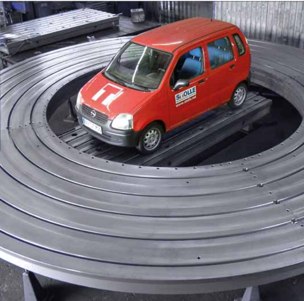
Turntable machining for ship propeller machining, 10,000 mm in diameter
