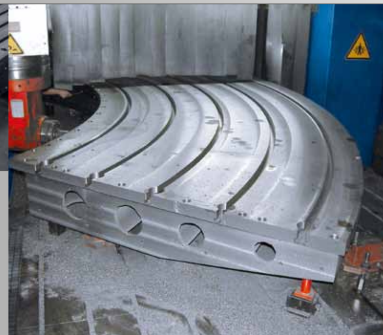
Segment of a turntable with a diameter of 10,000 mm
