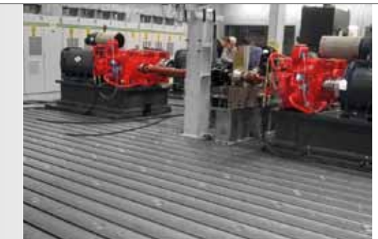
Test field for component tests Tooling plate size 14,000 x 10,000 mm durably connected with the seismic mass and designed with vibration isolation
