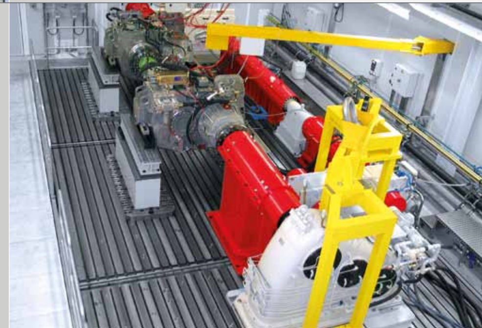
Large-scale transmission system test stand for ship transmission systems 15,000 x 8,000 mm
