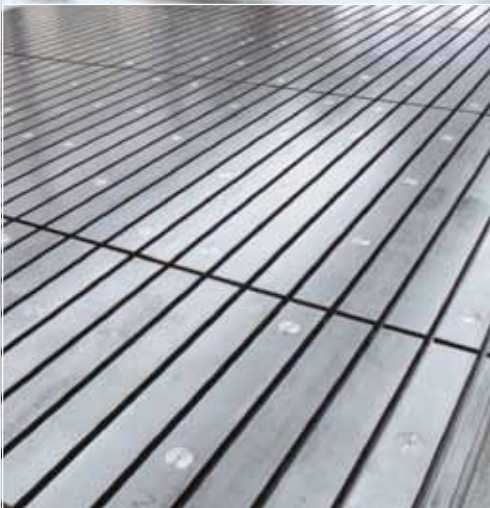
21,000 x 11,000-mm tooling plate
