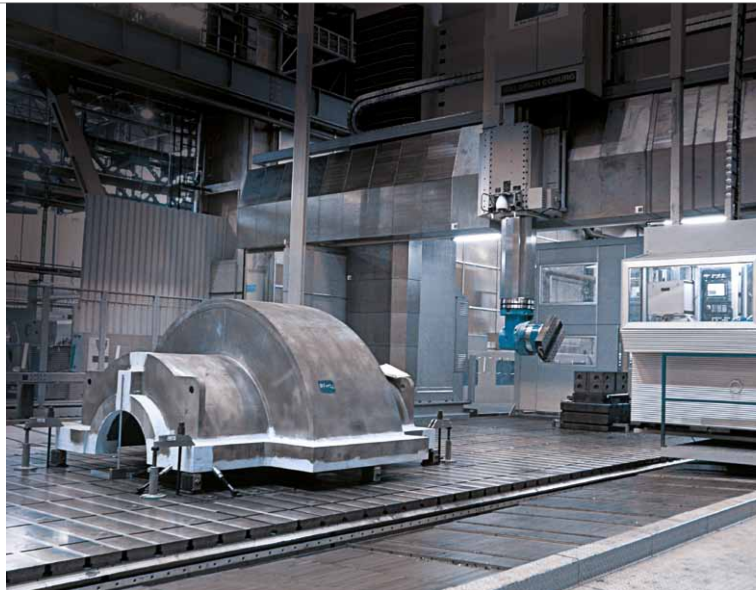
Large-scale processing centre using gantry construction with a STOLLE tooling plate field, 32,000 x 6,000 mm
