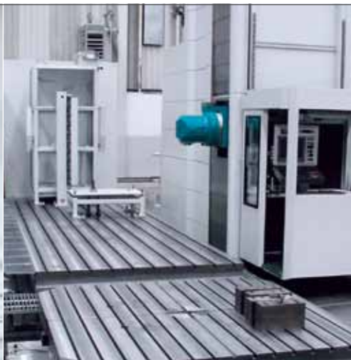
Tooling plate in a moving column milling machine
