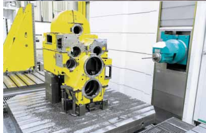
Large-scale processing centre using gantry construction with a STOLLE tooling plate field, 32,000 x 6,000 mm
