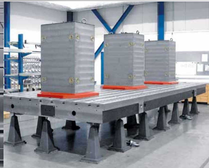
Clamping towers with zero-point clamping system
