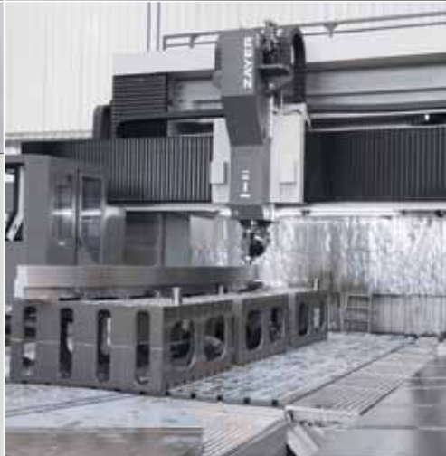
Tooling plate for a gantry machine
