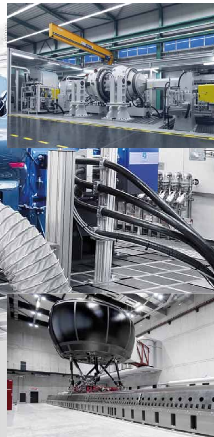
Driving simulator in Sindelfingen Air suspension of the hexapod on a base construction 31,000 mm long
