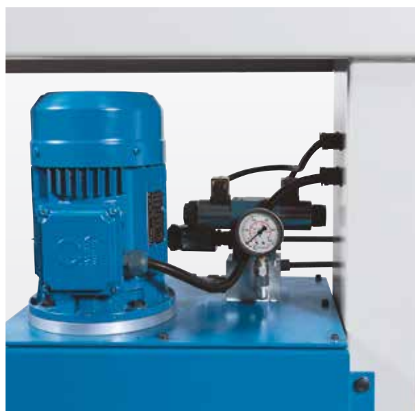
Compact hydraulic unit for powerful tube clamping
