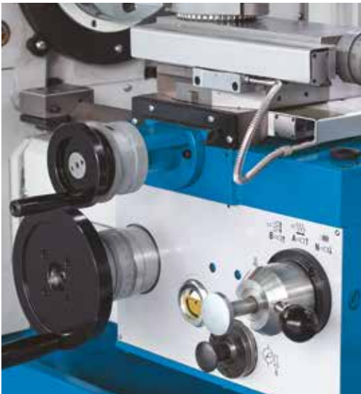
Central lubrication is integrated into the support for easy maintenance and handling
