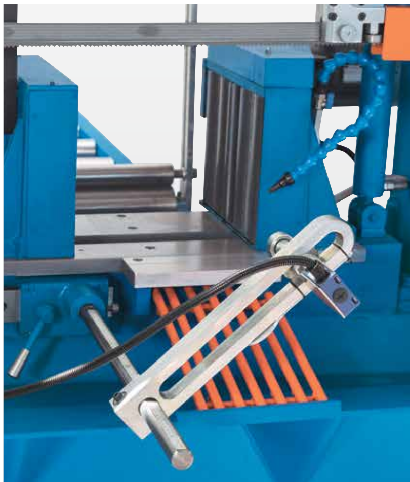
Driven feedrate rolls stop automatically when the material
