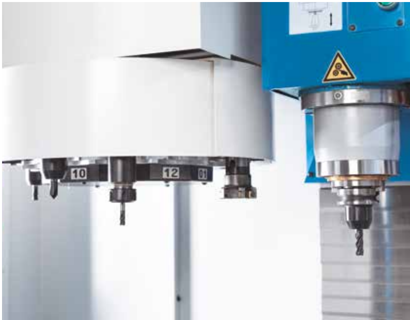
Rugged horizontal tool changer with 12 stations
