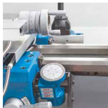
The thread gauge allows for resuming the thread after the apron nut for retrograde motion has been opened
