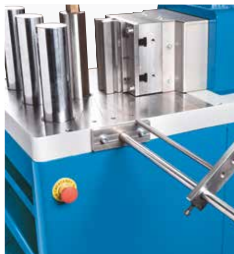
Manual side stop for batch production
