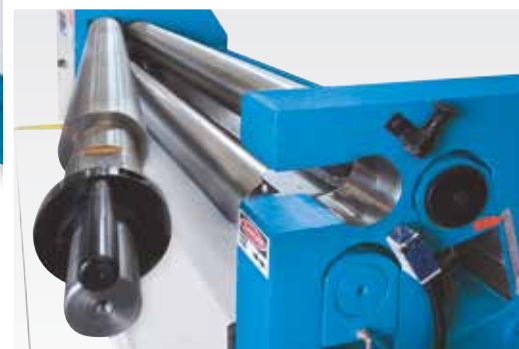
Upper roller can be swiveled out
