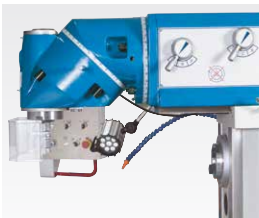
Universal cutter head, swivels on 2 planes
