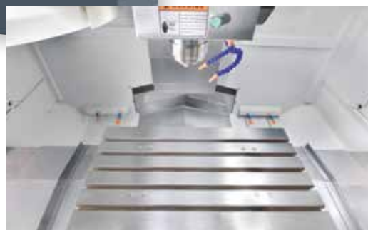
The guides in all axes are protected by robust stainless steel covers
