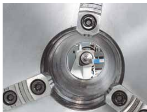
Spindle bores up to 225 mm
