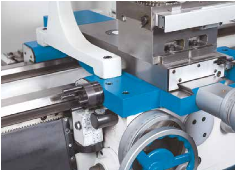
Stop spindle with 6 adjustable stops
