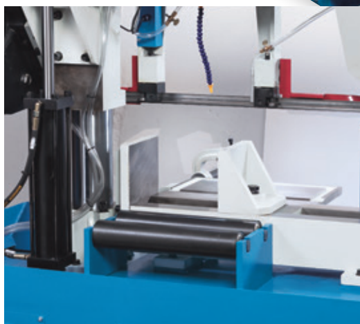
Roller support for easy material advancement
