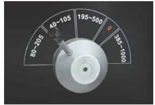
4 gear stages for high torque in the entire speed range
