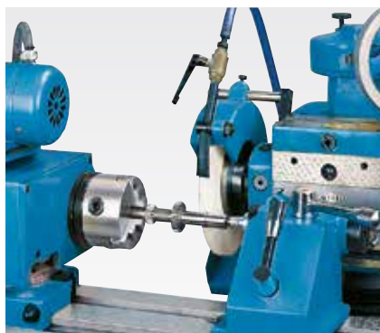
Outside cylindrical grinding for lengths up to 400 mm
