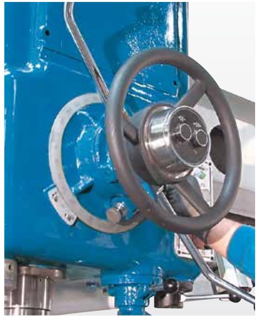
Depth stop with vernier scale
