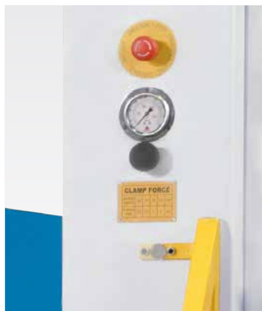
Adjustable upper die clamping pressure
