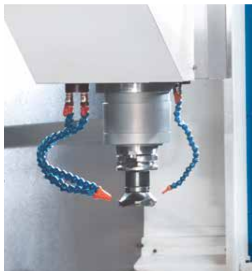
Spindle mount with cutter head
