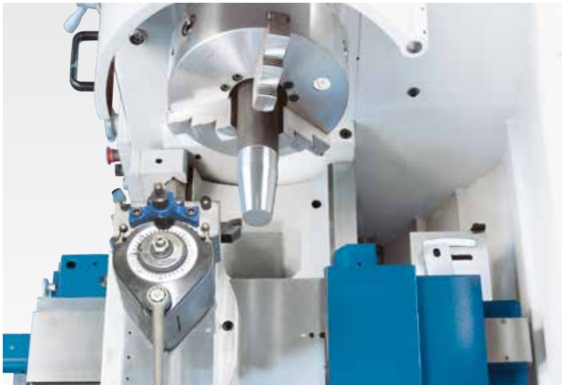
Taper turning unit is included
