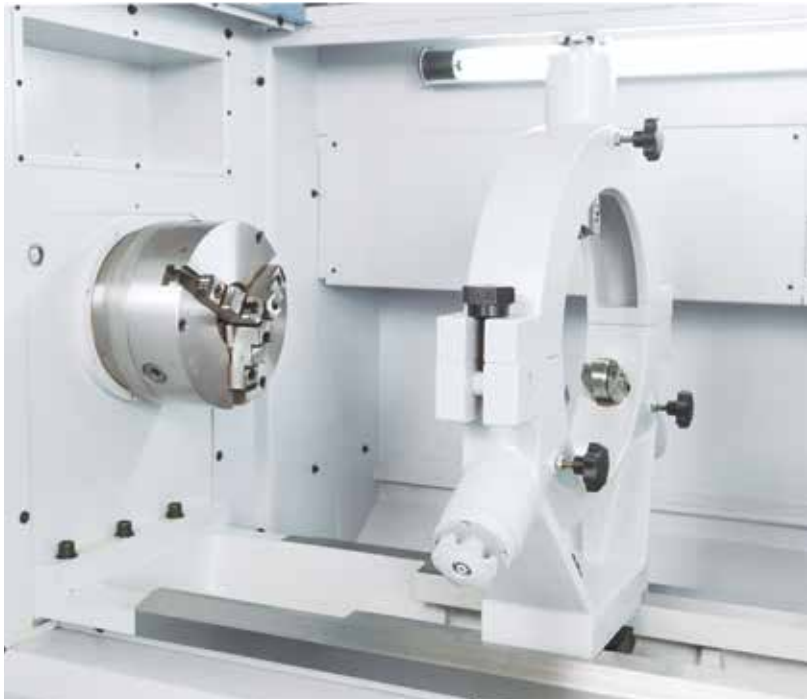
Option: steady rests up to 400 mm diameter
