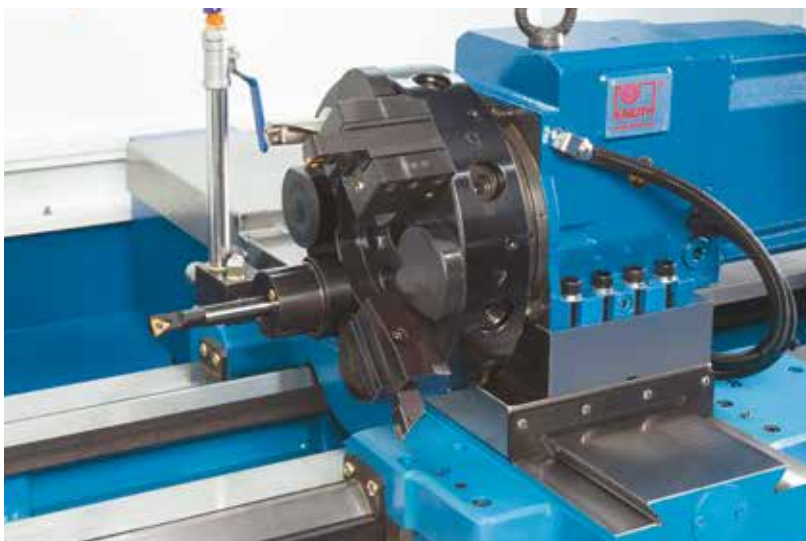
VDI 30 Tool Turret with 8 stations (Numturn 420 SI)
