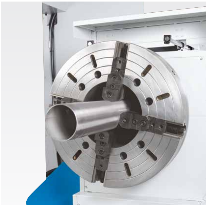
4-jaw chuck, at left side
