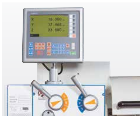
Positioning indicator on X-, Z- and Z1-axis
