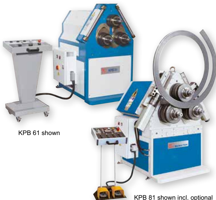
KPB 81 shown incl. optional accessories hydraulically controlled straightening rollers
