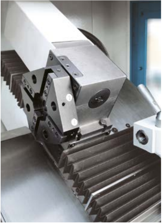
8-station tool turret with 4 tools per station for inside and outside turning
