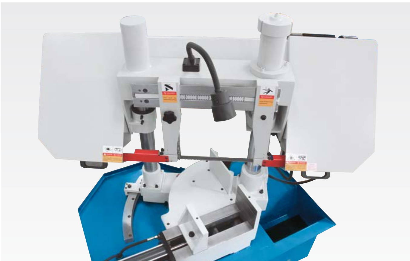
Rotating saw frame with dual-column guide
