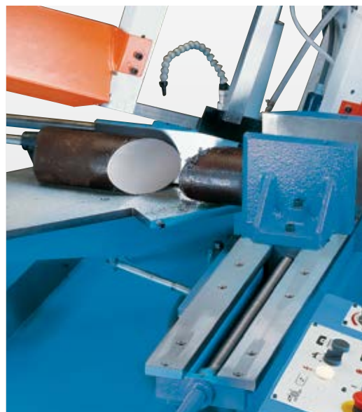
HB 320 BS: after cutting the sawframe is lifted automatically
