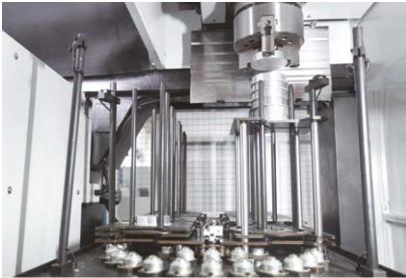
Workpiece storage with 8 stations
