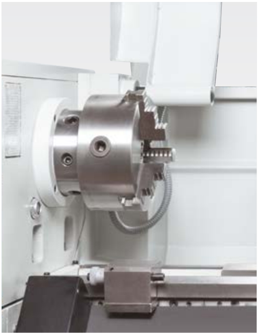
Micrometer bed stop ensures repeatability
