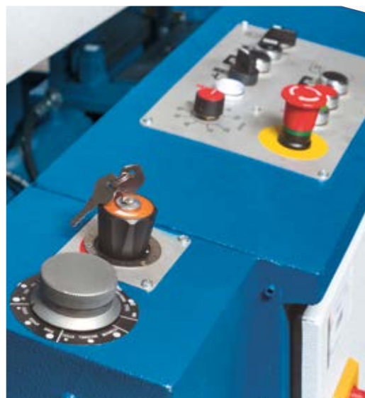
The constant pressure control (PAS) allows optimized feeding depending on material and profile type
