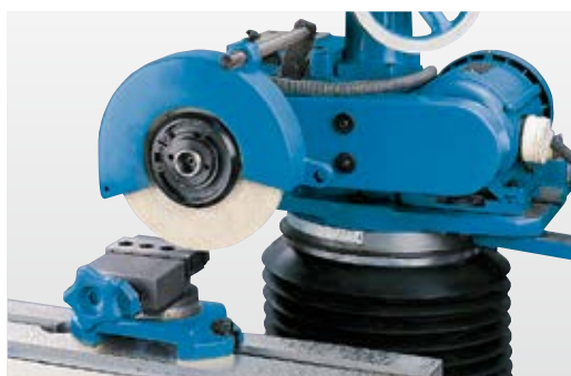
Surface grinder with angular adjustable vise
