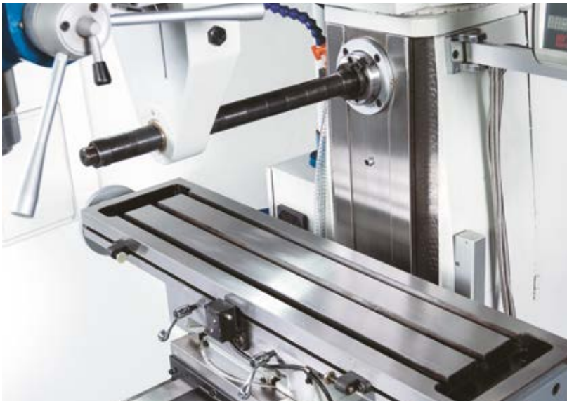
Solid top beam with outer arbor allows rigid mounting of long milling arbors
