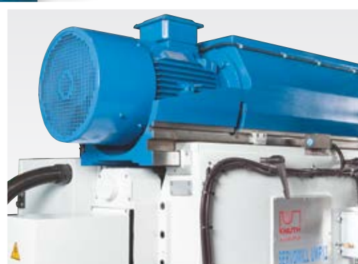
Powerful headstock drive with auxiliary gearbox (Servomill® UWF 12)
