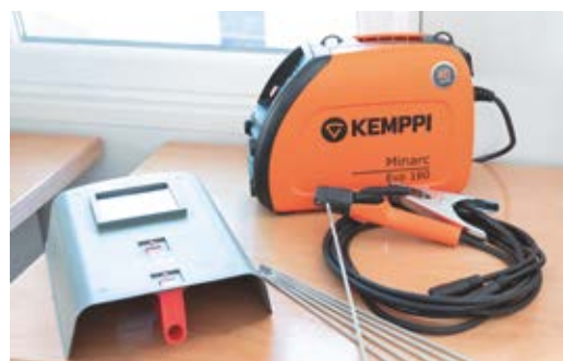
Compact welder, including face shield and electrodes
