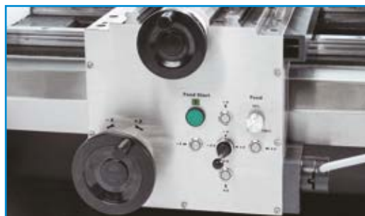
Electronic stops for X and Z axis
