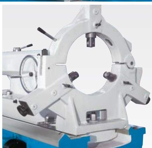
Steady rest with large capacity
