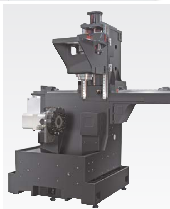
Mineral-casting machine frame with roller guide
