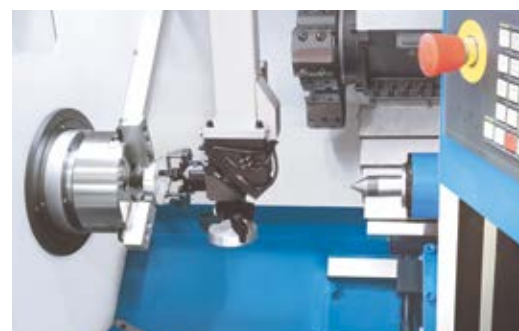
Dual grippers are provided for unloading and loading in one operation
