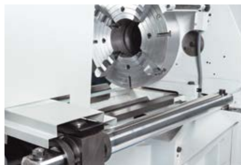
Taper turning unit is included
