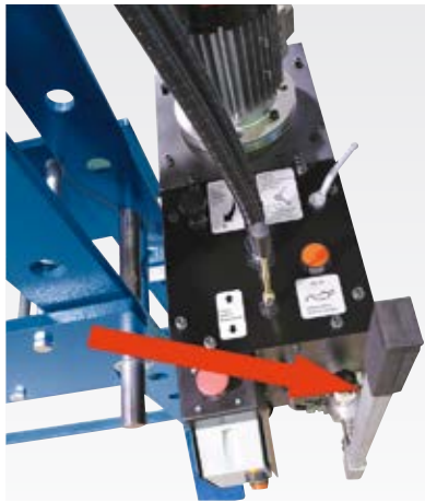
A hand pump is available for very delicate work
