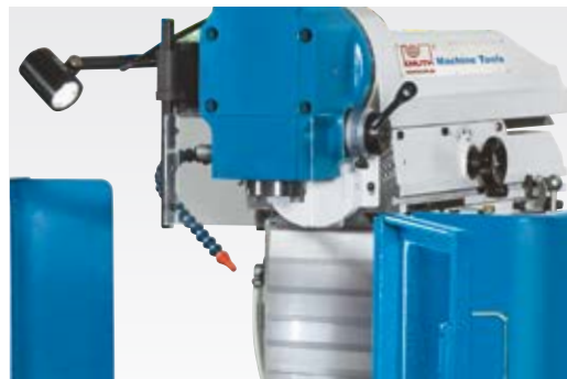
The main spindle drive is located centrally in the FPK 4
