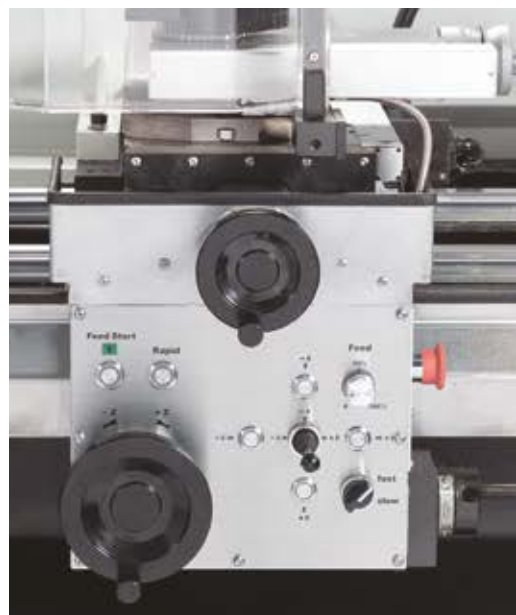
Servo drive technology – including "Teach-in" buttons that allow setting a limit stop at the current position
