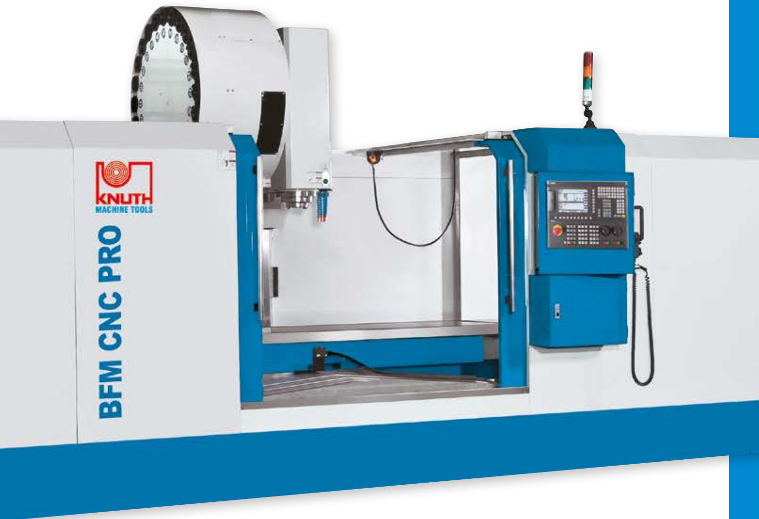
BFM CNC Pro shown with totally enclosed housing and chip conveyor
