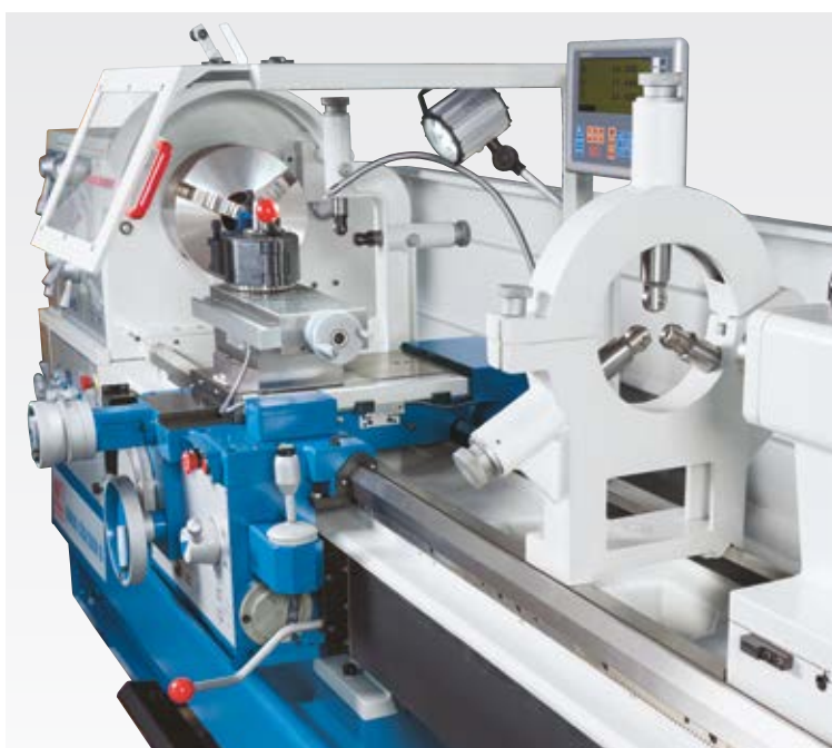
Rests ensure maximum precision when machining long workpieces
