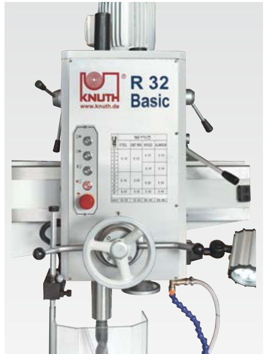
Hand-lever for quill feed is used to control the automatic feed
