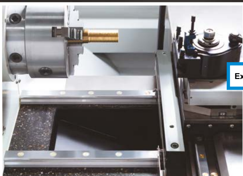
High-performance mineral casting machine frame with high-precision linear guides
