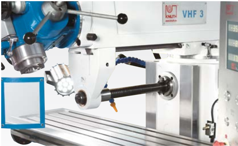
Horizontal milling spindle with outer arbor support for long milling arbors
