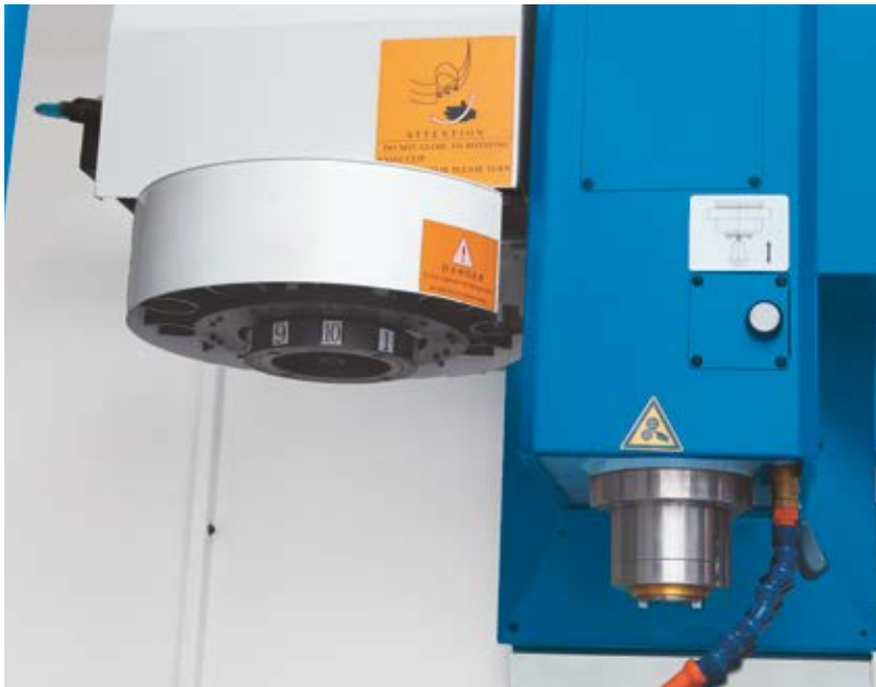
Rugged horizontal tool changer with 12 stations
