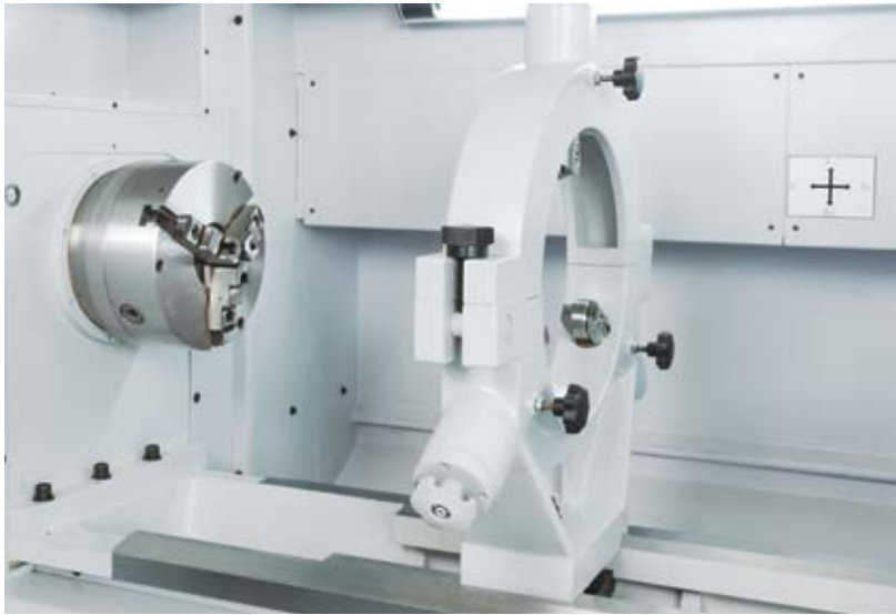
Option: steady rests up to 400 mm diameter
