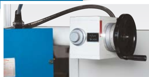
In automatic mode, the vertical feed increments can be preselected (VC models)
