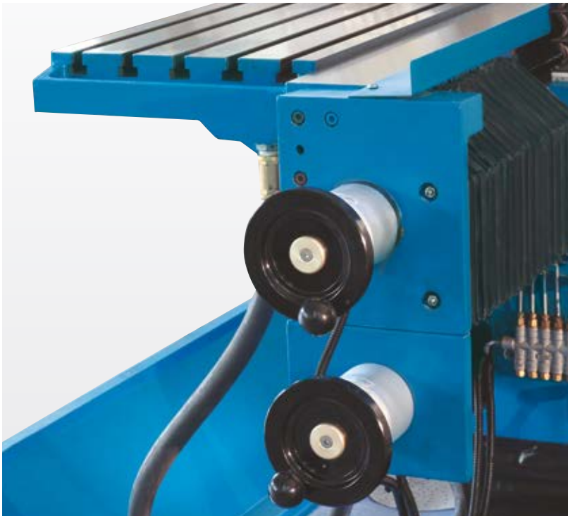
Micro-control via electronic hand-wheels - but handling and positioning just as with a conventional machine
