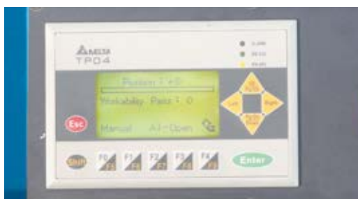
The rod magazine control can be configured at the user-friendly control panel
