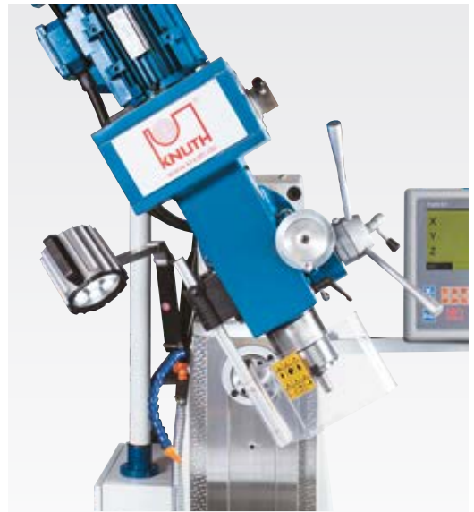
Swiveling cutter head with sliding quill
