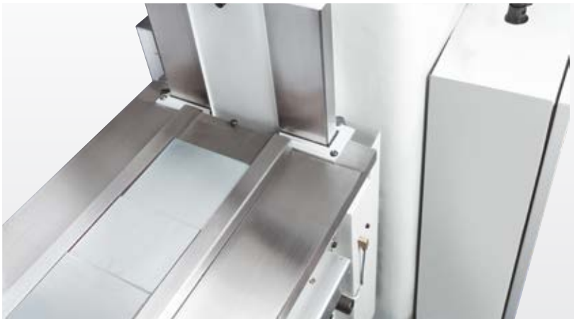
Wide, rigid box ways on Z and Y-axes
