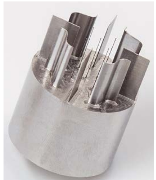
Machining time 4h20min (GEST 80), Pins Ø 5 x 0.2 mm, wall thickness 8 x 0.3 mm
