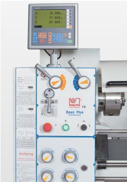
Positioning indicator on X, Z and Z1 axes
