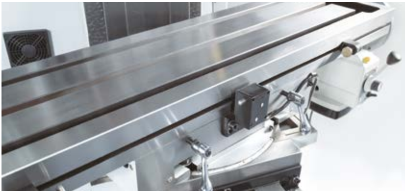
Cutter table swivels in X axis
