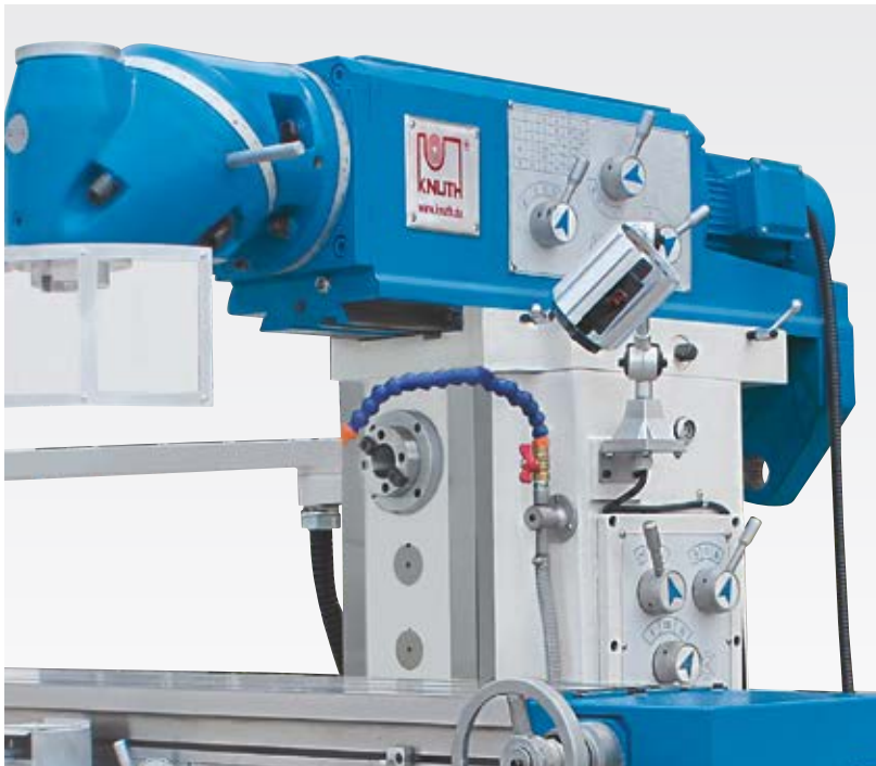
Vertical and horizontal spindle each have their separate drive
