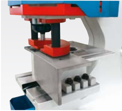
Hole punch station featuring large support table
