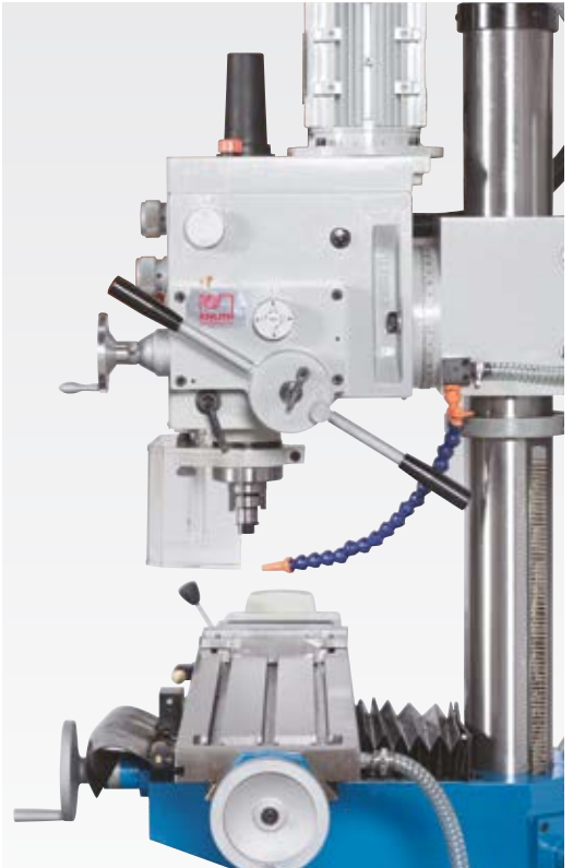
Automatic quill feed with 3-step gears
