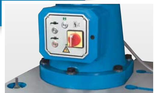
Rigid column base with central main switch
