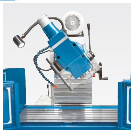
Angel-adjustable vertical cutter head with sliding quill
