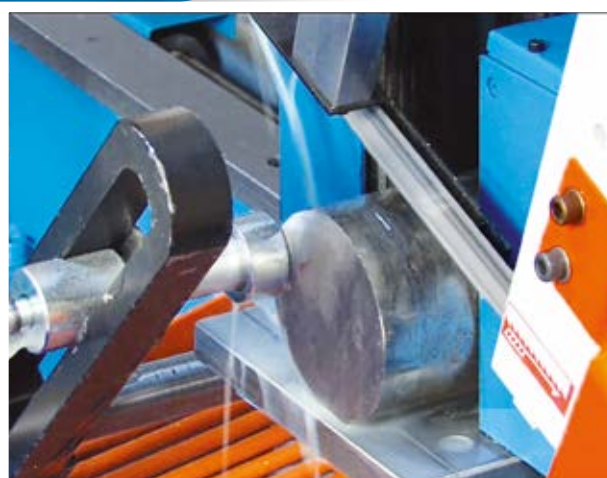
Automatic limitation of frame lift-off upon completion of the cut
