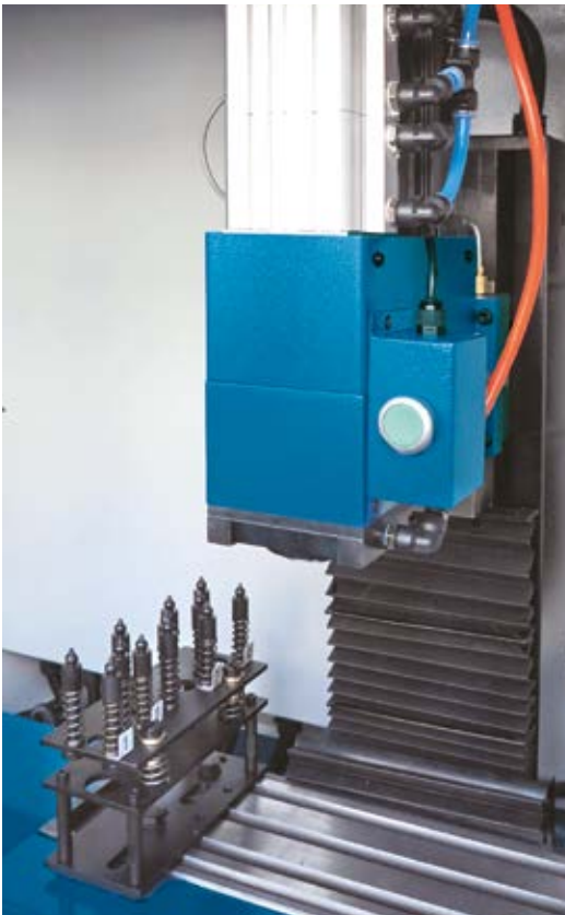
Pneumatic tool clamping
