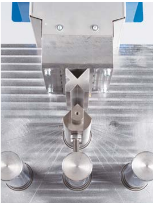
Angle lines are engraved in the work table for easy orientation
