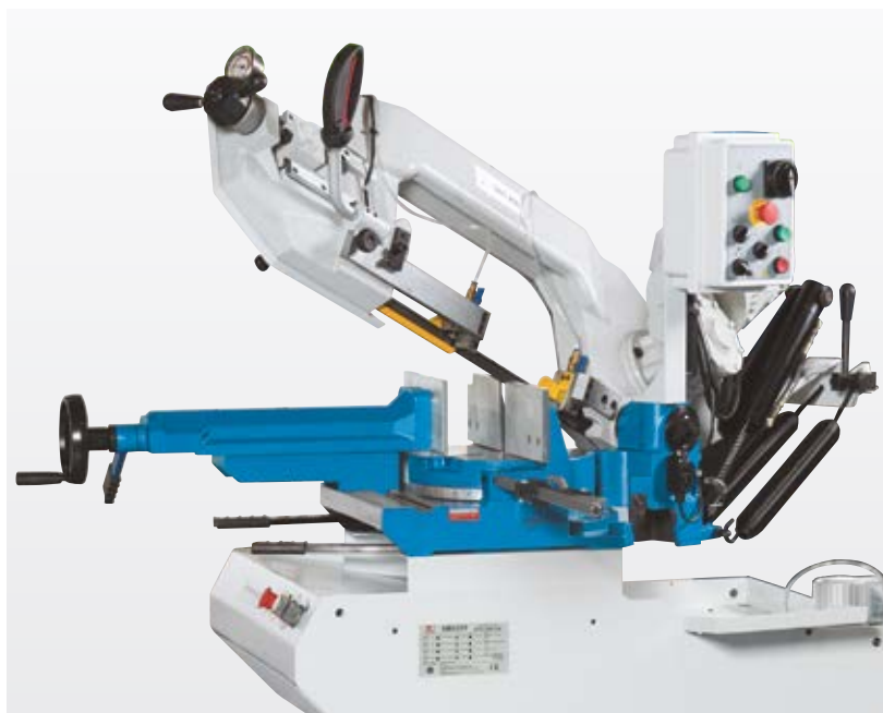
Saw frame with hydraulic or manual feed
