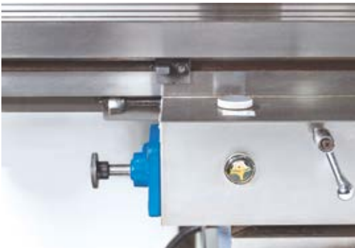
Integrated manual central lubrication
