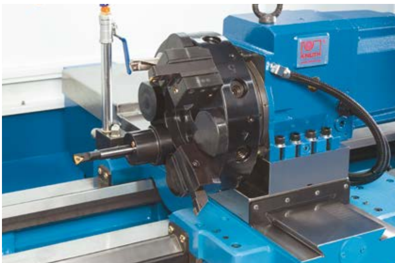
VDI 30 Tool Turret with 8 stations (Numturn 420)
