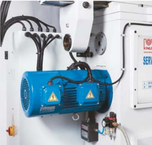
Powerful drive for horizontal spindle
