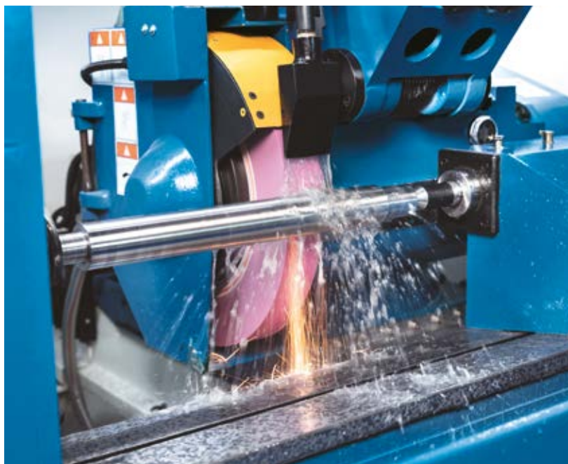
Easy programming of grinding cycles: Plunge-cut grinding, plunge-cut grinding with oscillation, and cylindrical grinding
