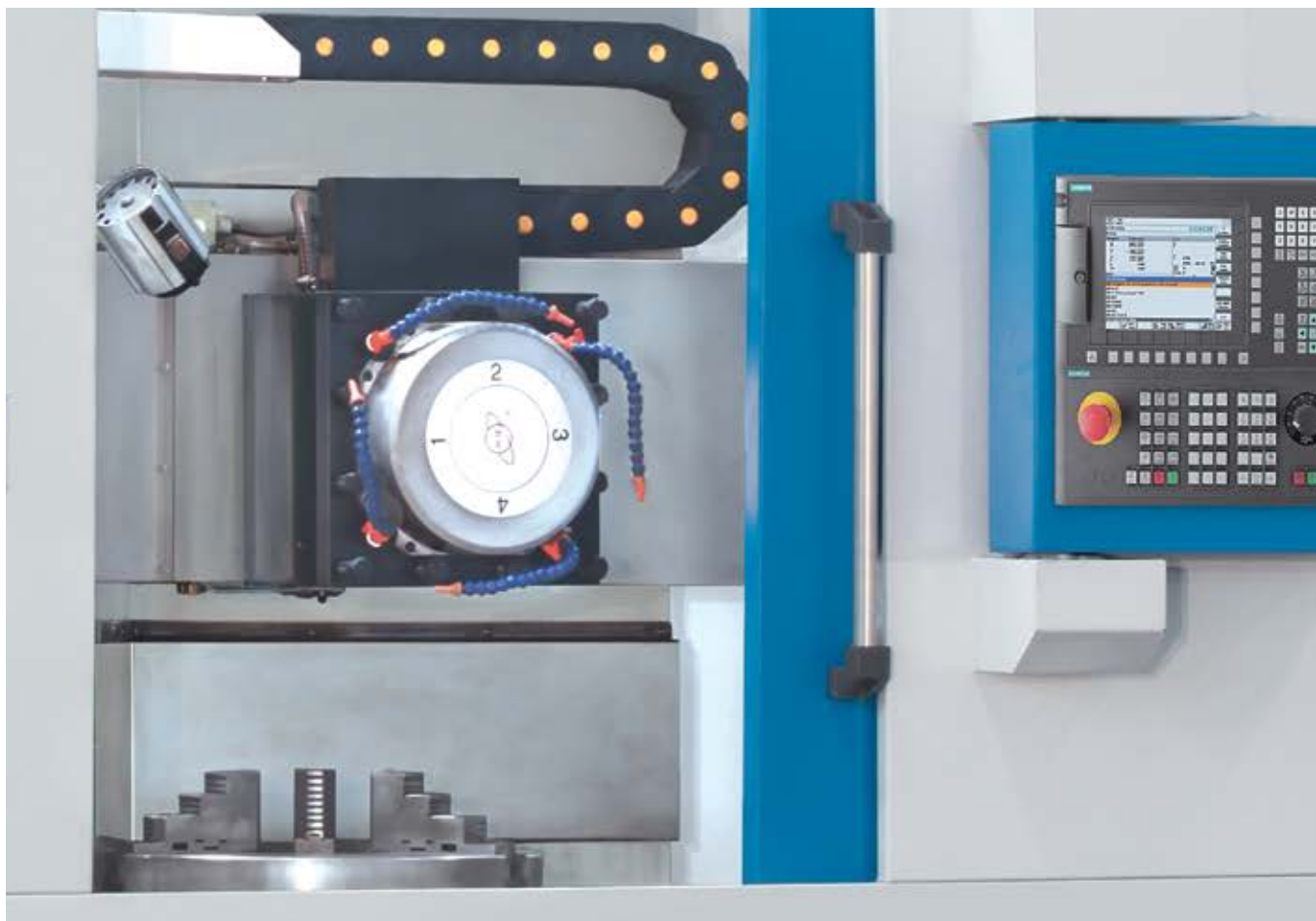
Rigid 4-station tool holder, 40 mm
