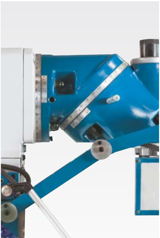
Cutter head swivels on 2 levels
