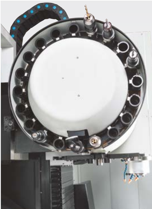
20-Station Tool Changer with twin-gripper arm
