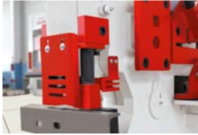
Notching station with safeguard
