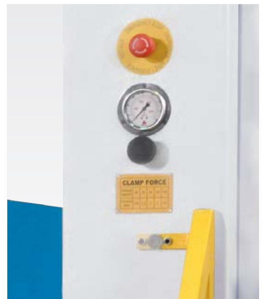
Adjustable upper die clamping pressure
