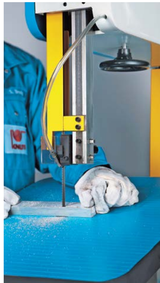
Precise saw blade guide can be adjusted to various blade widths
