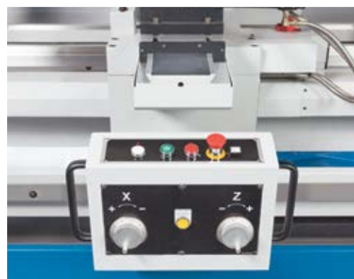
Compact control unit with electronic hand-wheels
