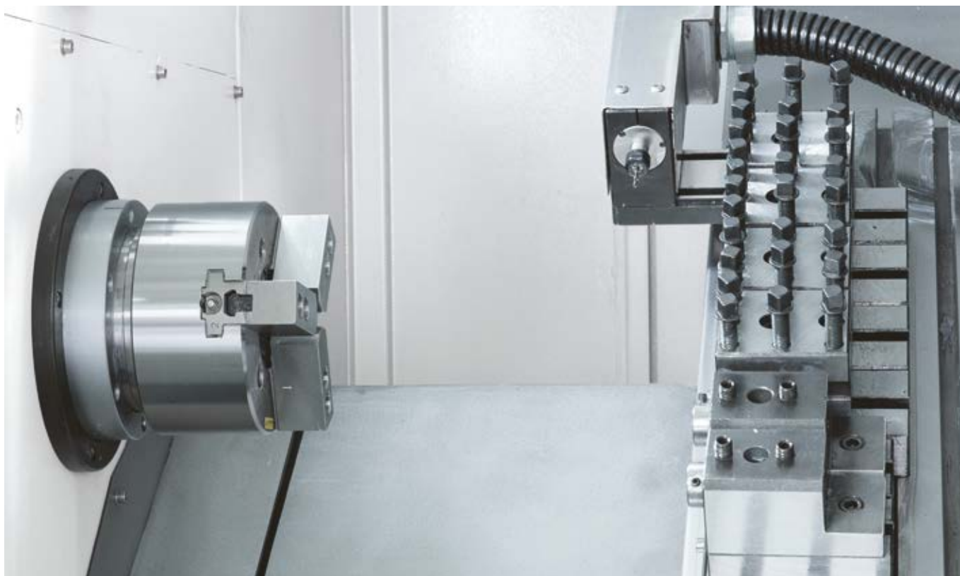
Linear tool changer with a radial driven tool (optional)
