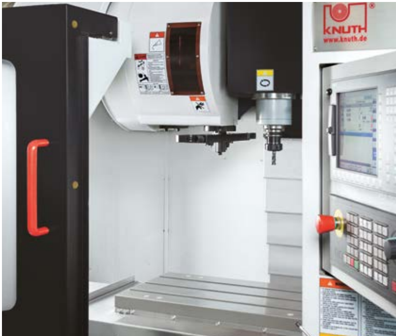
Dual-arm 16-station tool changer for quick and precise tool changes
