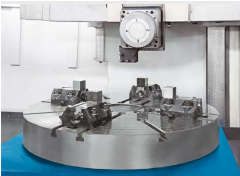
Face plate with 4-station tool changer
