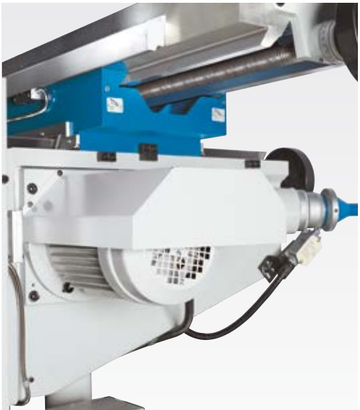
Rapid feed on Z axis with safety switch
