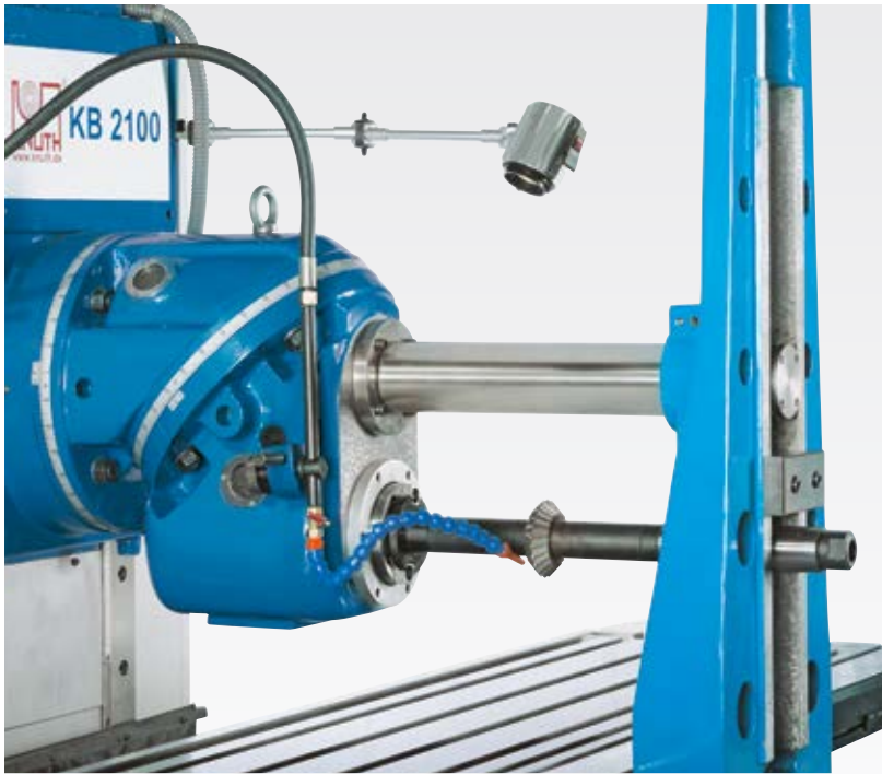
Rigid outer arbor system for long milling arbors
